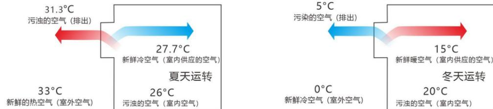
$$\text{全热交换效率}(\eta) = \frac{\text{新风空气焓值(HOA)} - \text{送风空气焓值(HSA)}}{\text{新风空气焓值(HOA)} - \text{室内回风空气焓值(HRA)}} \times 100\%$$
